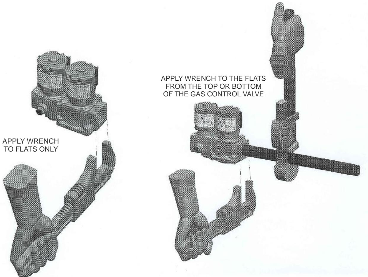
**Figure 5: Proper Use of Wrench on Gas Control**
