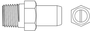
**Figure 3: Y99AX-1 (1/8-27 NPT) Pressure Test Fitting
