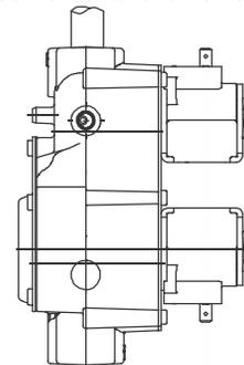
Vertical mounting may be 360° around its axis with the gas flow either up or down, but always in the direction of the arrow.
