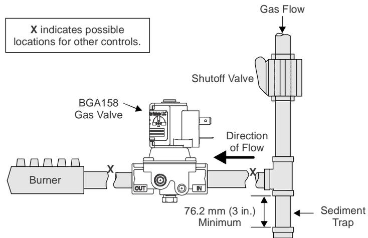
**Figure 5: Typical BGA158 Installation**
