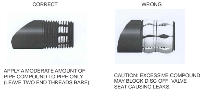
Figure 2: Use a Moderate Amount of Pipe Compound
