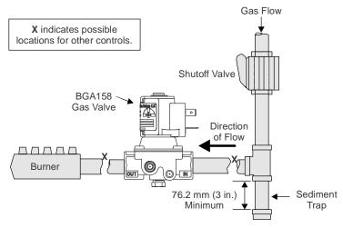
Figure 3: Typical BGA158 Installation
