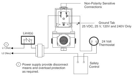
Figure 2: 3-Tab Electrical Connections
