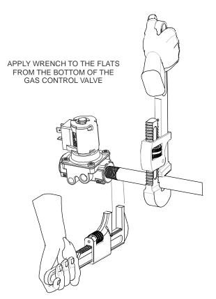
Figure 3: Proper Use of Wrench on Gas Control \*\*DO NOT USE THE COIL FOR LEVERAGE
