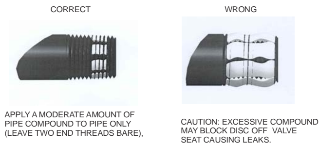
Figure 2: Use a Moderate Amount of Pipe Compound
